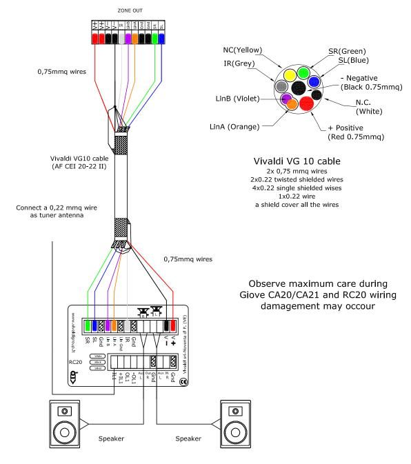
Noise rejecting and correct operating of Giove CA20 are guaranteed only by using VG10 cable. Other cables may not allow correct operation of CA20-RC20 systems.
