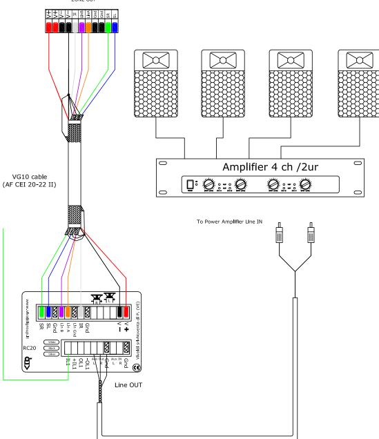
RC20 AUX-Out can drive a booster amplifier to cover large areas, it is also possible to connect speakers on the RC20 speaker socket.
