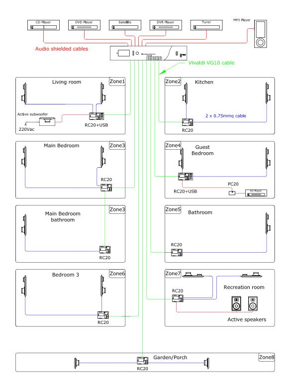
On the example shown a CA20 is fitted with 8 zones (RC20) plus a subzone in mirror mode with the main bedroom.
