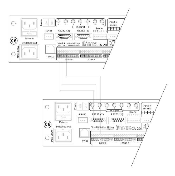
Following this scheme it is possible to use two or more main units, using the IR signals and the switched outputs together.
