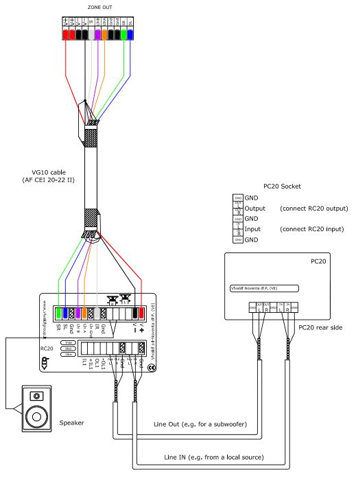
PC20 is a module designed to locate RC20 AUX In and AUX Out to a more convenient position. PC20 has 4 RCA plugs on its front panel and must be connected to the smallest RC20 socket, using high quality well shielded audio cable, such as microphone cable or similar.
