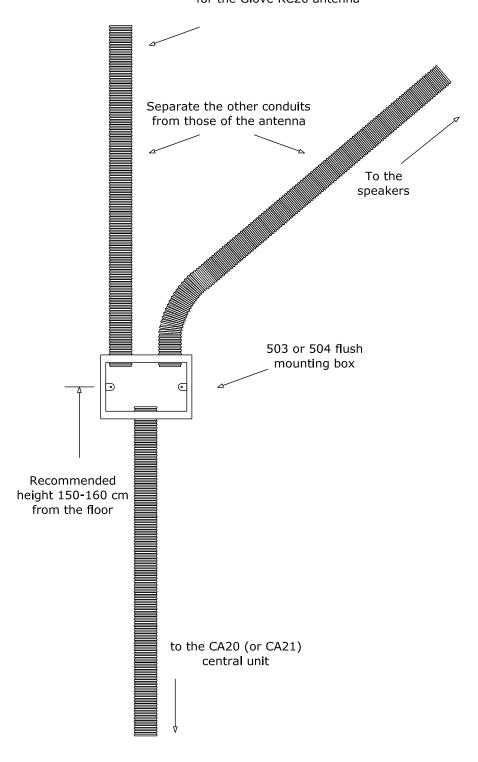
Here we show a typical example of in-wall set up for an RC20.
