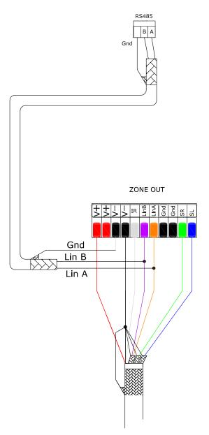
Connect the Giove CA3MKII to a Giove CA20/CA21 zone socket, using an empty socket or connecting the CA3MKII in parallel to a RC20 cable as shown.
