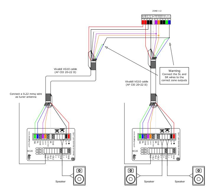
Follow this scheme to connect more RC20s in parallel, to a CA21 (Mirror or Slave configuration). This scheme is an example; it shows how to connect 2 RC20s to the first Zone of a CA21 Pay close attention to SL and SR signals, they represent the only difference between the CA20 and CA21 Slave/Mirror wiring.
