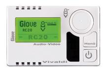
Switch the RC20 On or Off with a single, short pressing of  $\overset{\mbox{\ }}{\mbox{\ }}$  key.
