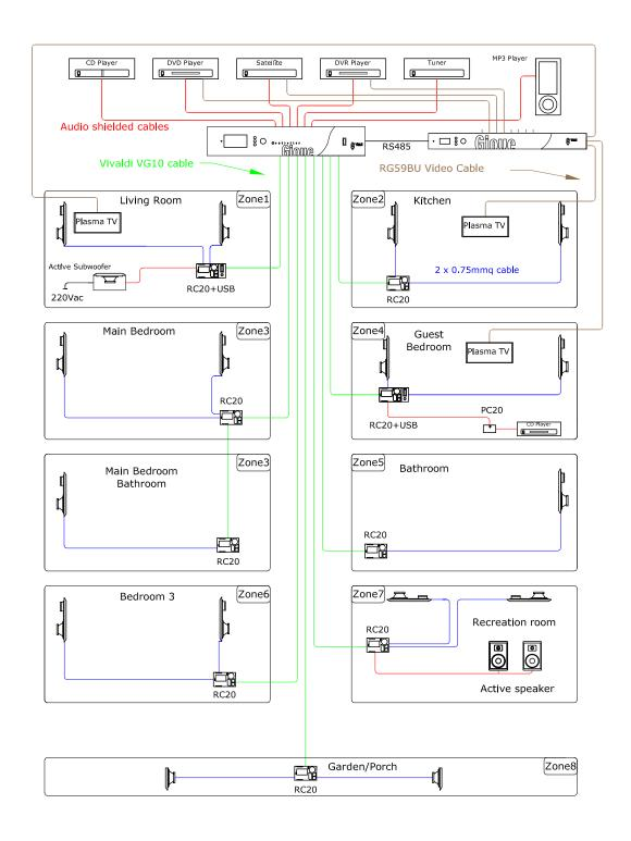
In this example video distribution is added to the tradional audio multiroom distribution. In this way it is possible to have the use of video sources, other than audio. Selection of video sources is totally automatic, for example selecting the DVD on the RC20 both the audio and video signals will be set and it will be possible to see the video on a TV and listen to the audio on the loudspeaker wired to the RC20.
