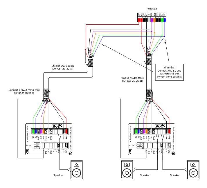
Follow this scheme to connect more RC20s in parallel, to a CA20 (Mirror or Slave configuration). It is not necessary to route all the cables to the main unit, in many cases it can be more convenient to wire an RC20 to another than going to the main unit with only one cable (see examples on pages 26 e 27, main bedroom and bathroom).
