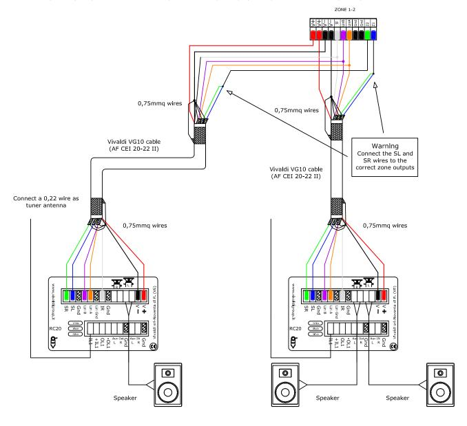
Giove CA21 (16 zones) wiring. Observe maximum attention in wiring. RC20 controllers must be set in accordance with the zones where they are connected (refer to page 16 for detailed instructions). Max 16 RC20s for every Giove CA21 main unit can be connected. It is possible to connect up to 40 Giove RC20s to a Giove CA21 system, but it is necassary to use a booster supply (Giove AL10) to connect more than 16 RC20s to such a system.
