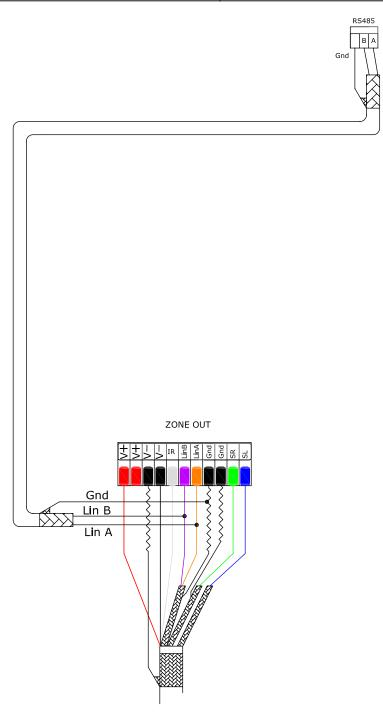
Connect the Giove CA3MKII to a Giove CA20/CA21 zone socket, using an empty socket or connecting the CA3MKII in parallel to a RC20 cable as shown.
