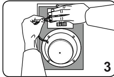
Please connect the speaker cable to the screw clamps. Ensure that the polarity is correct.
