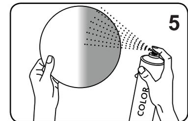
The grille cover of the InWall/InCeiling systems can simply be coated with regular paint. If the grille cover of your system comes with an additional coating this must be removed before painting.
