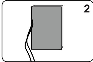
When laying loudspeaker cable from amplifier to installation point, be sure that the cable ends about 30 cm (12") beyond the wall cutout.
