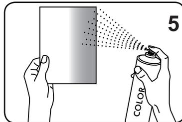
The grille cover of the InWall/InCeiling systems can simply be coated with regular paint. If the grille cover of your system comes with an additional coating this must be removed before painting.
