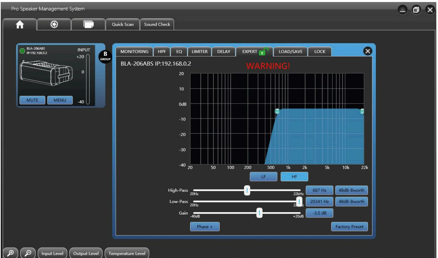
A crossover is used to divide the broadband signal into separate frequency bands. This allows each driver in a speaker system to be operated within its optimal frequency range. Using active crossover increase the efficiency of each driver but also of the amplifier by lowering the intermodulation distortion.
